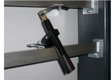
FIX laser, manually adjustable to indicate saw blade position
